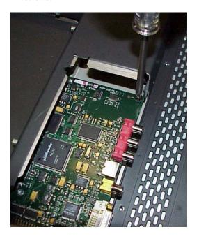
9. Slide the DVI or SDI replacement cover panel into place. Press down gently on the insertion end of the panel to help the tabs insert in the slots.
